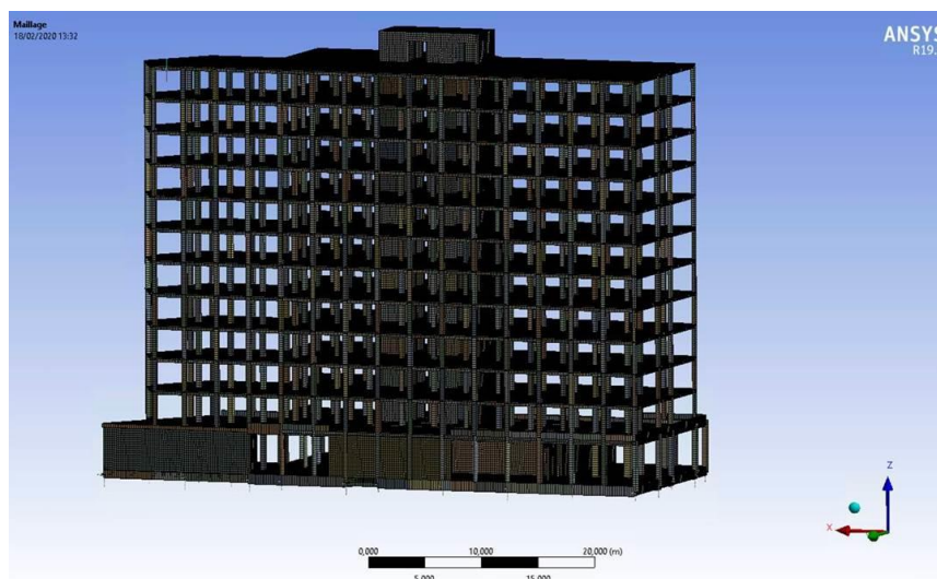
Figure 5: Ansys model of the Treed-It building by CSTB, using beam elements for the columns and beams and shells for the slabs and the concrete core.
